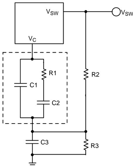
Figure 38. Technique for Increasing Slope Compensation
