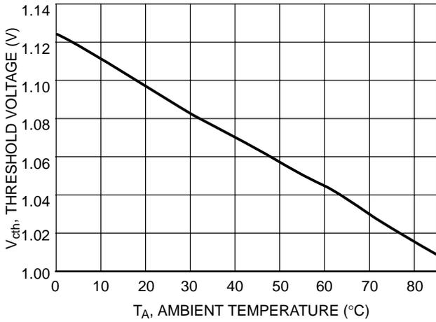
**Figure 15.  $V_C$  Threshold Voltage versus Temperature**
