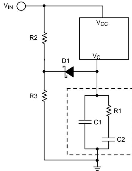
**Figure 36. Current Limiting using a Diode Clamp**
