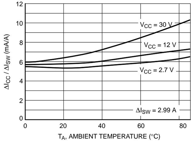
**Figure 4.  $\Delta I_{CC} / \Delta I_{SW}$  versus Temperature**
