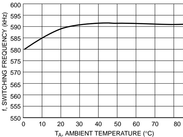
**Figure 7. Switching Frequency versus Temperature (NCP1444/5 Only)**
