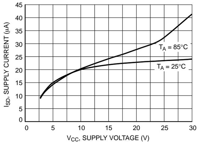
**Figure 20. Supply Current versus Supply Voltage During Shutdown**
