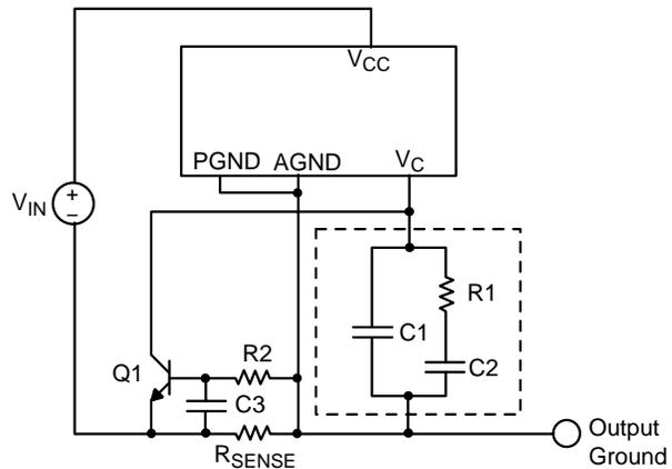
**Figure 37. Current Limiting using a Current Sense Resistor**
