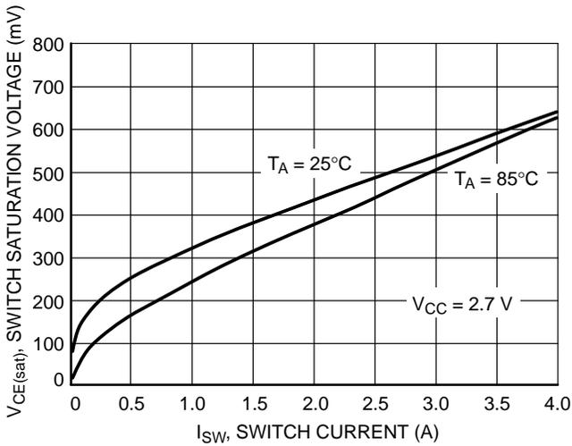
**Figure 5. Switch Saturation Voltage versus Switch Current**
