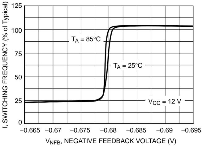
**Figure 9. Switching Frequency versus Negative Feedback Voltage**
