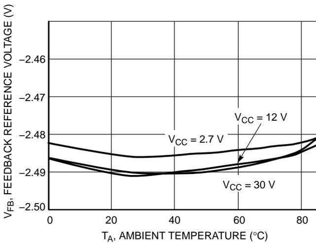
**Figure 11. Feedback Reference Voltage versus Temperature (NCP1443/5 Only)**
