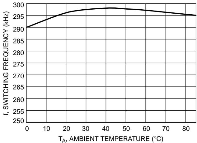
**Figure 6. Switching Frequency versus Temperature (NCP1442/3 Only)**
