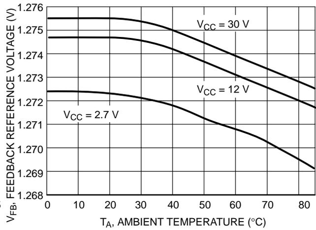
**Figure 10. Feedback Reference Voltage versus Temperature (NCP1442/4 Only)**
