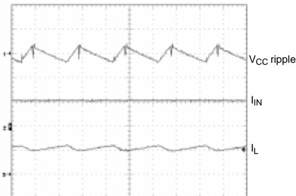
Figure 33. Boost Input Voltage and Current Ripple Waveforms
