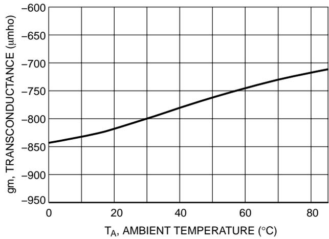
**Figure 22. Negative Error Amplifier Transconductance versus Temperature**
