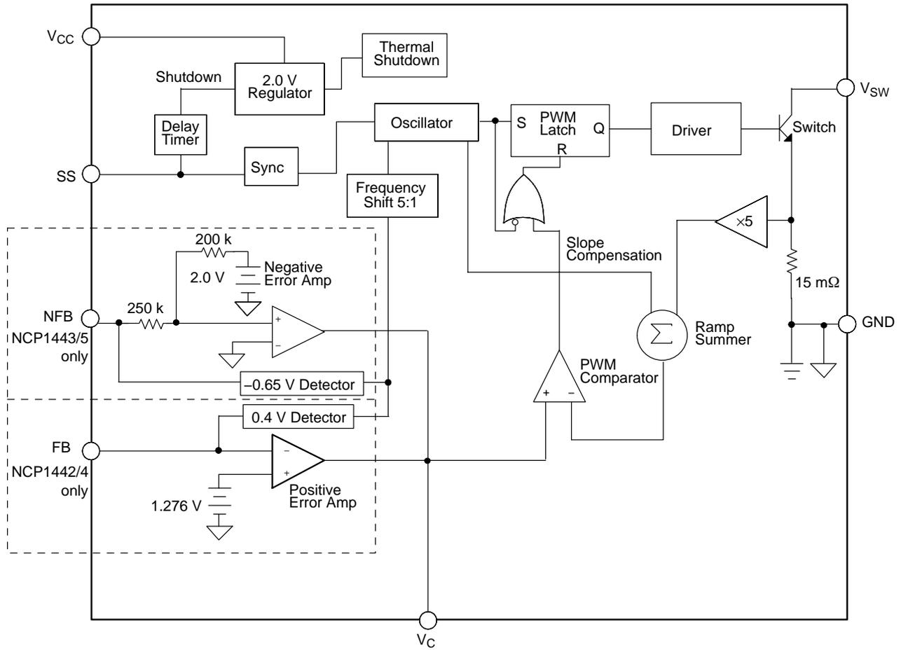
Figure 2. Block Diagram
