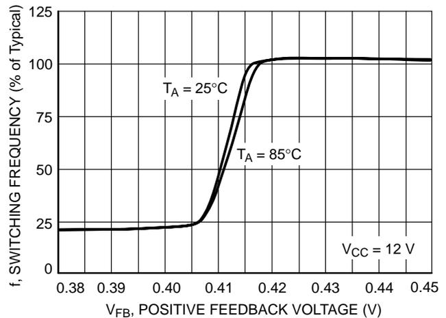
**Figure 8. Switching Frequency versus Positive Feedback Voltage**
