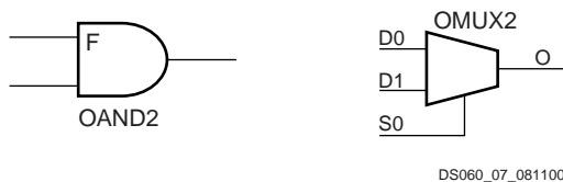
Figure 7: AND and MUX Symbols in Spartan-XL IOB
