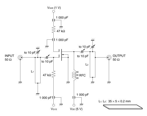
$V_{DS} = 5 \text{ V}, V_{G2S} = 1 \text{ V}, I_{D} = 10 \text{ mA}$
