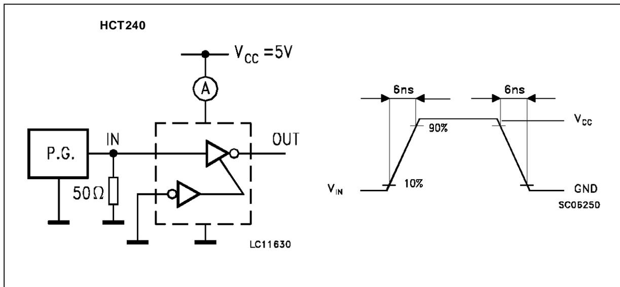
SWITCHING CHARACTERISTICS TEST WAVEFORM
