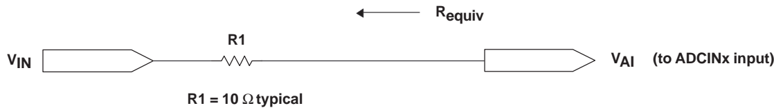
Figure 31. Typical ADC Input Pin Circuit
