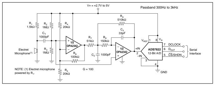
FIGURE 7. Speech Bandpass Filtered Data Acquisition System.
