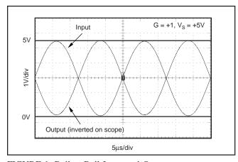
FIGURE 1. Rail-to-Rail Input and Output.
