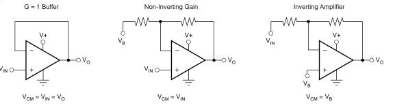
FIGURE 3. Design Optimization with Rail-to-Rail Input Op Amps.
