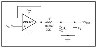
FIGURE 5. Series Resistor in Unity-Gain Configuration Improves Capacitive Load Drive.
