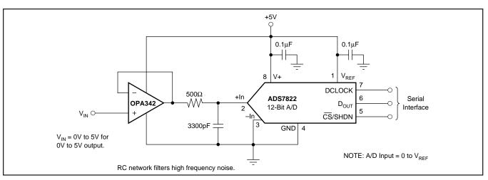
FIGURE 6. OPA342 in Noninverting Configuration Driving ADS7822.
