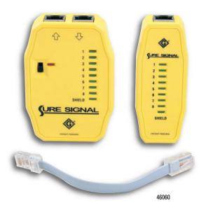
Designed for cable installers and communications technicians for testing four-pair data/voice cable links terminated with standard, modular eight-position RJ45-style jacks.
