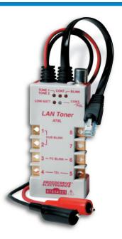
The LAN Toner is designed for the network installation and maintenance professional and can be used on any wiring system including datacom, telecom, security/alarm, audio and CATV.
