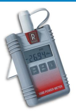
Suitable for power measurements on high power single-mode and DWDM fiber optic systems.
