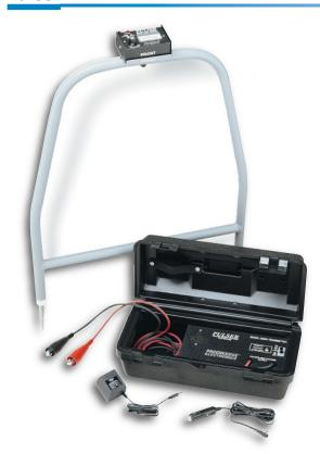
Identifies the exact location of even the smallest breaks in insulation by "pulsing" a high-voltage signal that radiates into the earth at the location of the faults. With the A-frame mounted receiver, a visual analog meter points the way to the source of the voltage.
