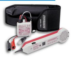
Used to identify single conductors or cables within a bundle, at a crossconnect point or at remote ends.
