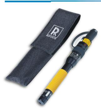
Pinpoints cable breaks and bad connections in both single-mode and multimode fiber.
