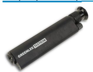
High-powered microscope is used to check a connector's endface for excess epoxy, core or cladding chips or other irregularities that degrade optical performance of the connector.
