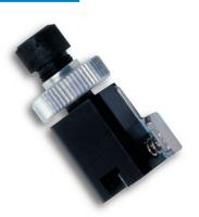
Allows temporary connection of 125 micron multimode or single-mode fiber to measuring equipment such as Sources, Optical Power Meters and Fault Locators with an FC-style connector. Connection to other common fiber optic connector styles can be accomplished with a hybrid test jumper.
