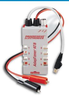
The AT Tone Generator makes it simple to test continuity, polarity, send tone and even supply talk battery to any configuration of pairs in 8-position modular jacks and plugs.
