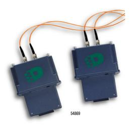
Converts any LANcat® System 5 or System 6 into a precision multimode optical loss test set.
