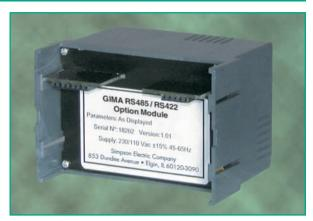
This Options Module may be configured as RS485 or RS422 providing 2 or 4-wire communications over distances up to 3/4 mile. Data rates of 4800, 9600 or 19200 baud may be selected to suit system requirements.
