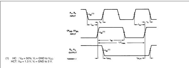
Fig.7 Waveforms showing the  $A_n$ ,  $B_n$  to  $CP_{AB}$ ,  $CP_{BA}$  set-up and hold times, clock  $CP_{AB}$ ,  $CP_{BA}$  pulse width, maximum clock pulse frequency and the  $CP_{AB}$ ,  $CP_{BA}$  to output  $B_n$ ,  $A_n$  propagation delays.
