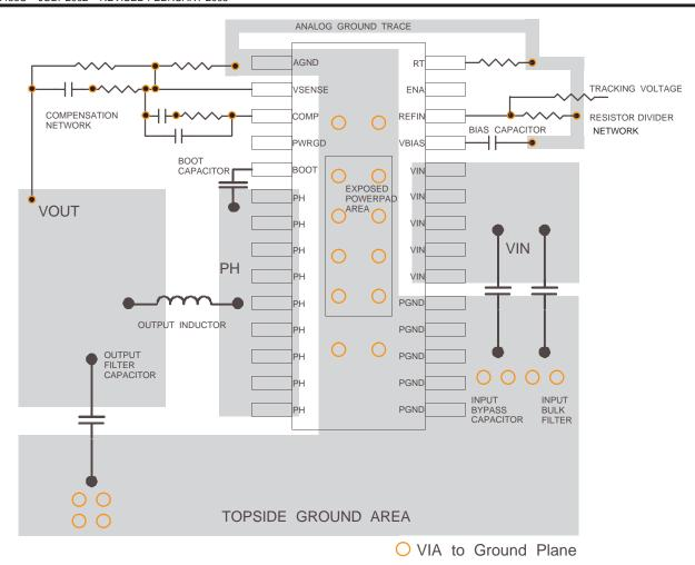
Figure 8. TPS54872 PCB Layout
