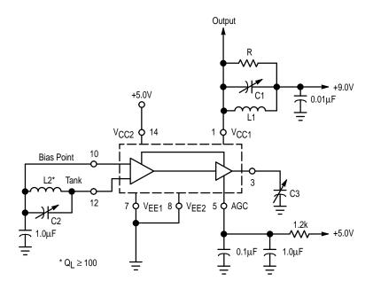
Figure 12. Circuit Used for Collector Output Operation
