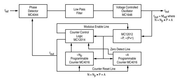
Figure 9. Typical Frequency Synthesizer Application
