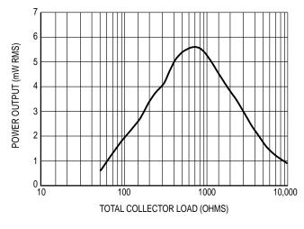
See test circuit, Figure 12, f = 100MHz C3 = 3.0–35pF Collector Tank L1 =  $0.22\mu H$  C1 = 1.0–7.0pF R =  $50\Omega$ – $10k\Omega$  Rp of L1 and C1 =  $11k\Omega$  @ 100MHz Resonance Oscillator Tank L2 = 4 turns #20 AWG 3/16" ID C2 = 1.0–7.0pF
