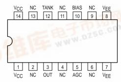
Pin assignment is for Dual–in–Line Package.
