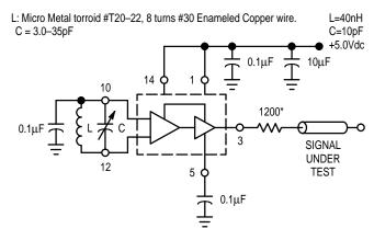
The 1200 ohm resistor and the scope termination impedance constitute a 25:1 attenuator probe. Coax shall be CT–075–50 or equivalent.
