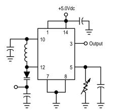
Figure 10. Method of Obtaining a Sine-Wave Output
