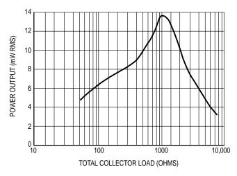
See test circuit, Figure 12, f = 10MHz C3 = 470pF Collector Tank L1 =  $2.7\mu H$  C1 = 24–200pF R =  $50\Omega$ – $10k\Omega$  Rp of L1 and C1 =  $6.8k\Omega$  @ 10MHz Resonance Oscillator Tank L2 =  $2.7\mu H$  C2 = 16–150pF
