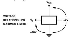
CAUTION: Stresses above those listed in "Absolute Maximum Ratings" may cause permanent damage to the device. This is a stress only rating and operation of the device at these or any other conditions above those indicated in the operational sections of this specification is not implied.
