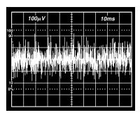
Figure 11. 10 Hz to 10 kHz Wideband Noise
