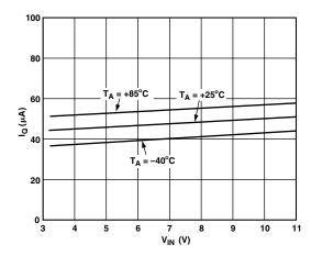
Figure 7. Typical Supply Current over Temperature
