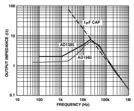
Figure 8b. Output Impedance vs. Frequency
