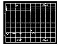
Figure 15. Load Transient Response (0 mA to -1 mA Load)
