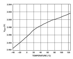
Figure 4. Output Voltage vs. Temperature
