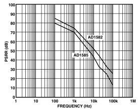
Figure 9b. Ripple Rejection vs. Frequency
