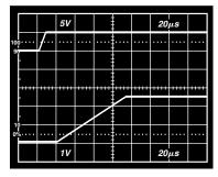
Figure 12b. Turn-On Characteristics
