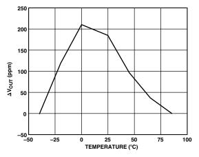
Figure 5. Residual Drift Error
