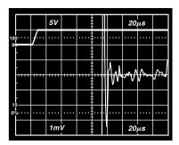
Figure 12c. Turn-On Settling
