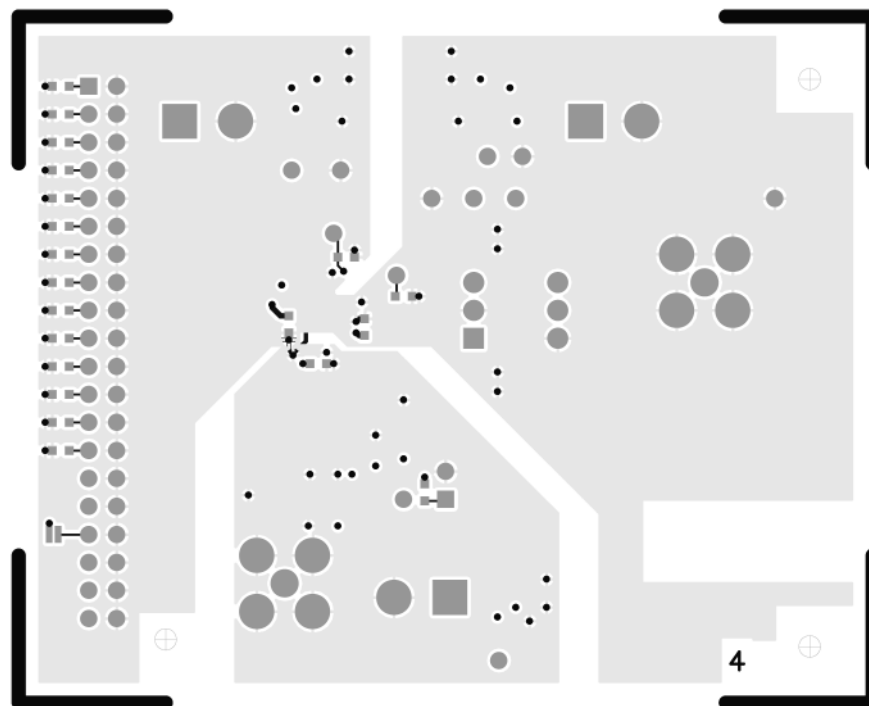
Figure 31. LFCSP Evaluation Board Layout—Secondary Side
