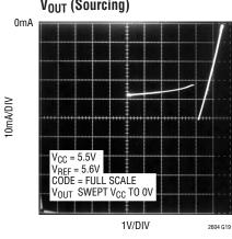
Short-Circuit Output Current vs V<sub>OUT</sub> (Sourcing)
