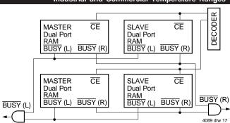
Figure 3. Busy and chip enable routing for both width and depth expansion with IDT7034 RAMs.
