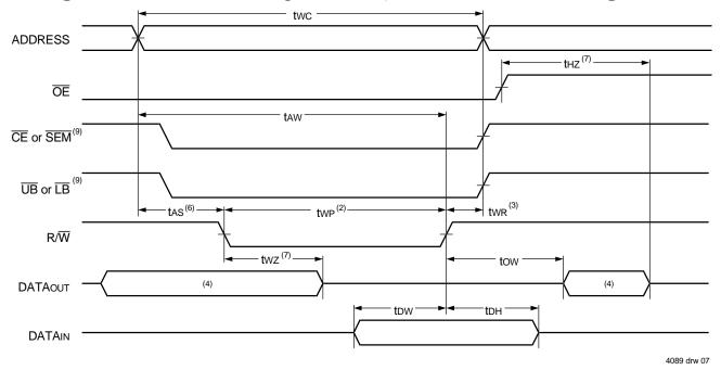
Timing Waveform of Write Cycle No. 2, CE, UB, LB Controlled Timing<sup>(1,5)</sup>
