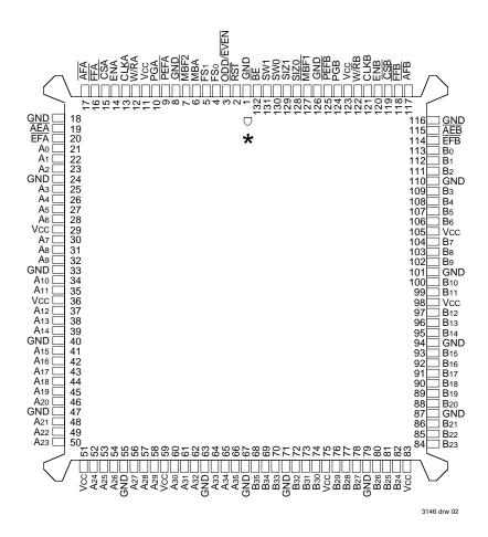
Electrical pin 1 in center of beveled edge. Pin 1 identifier in corner.
