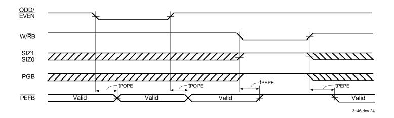
Figure 24. ODD/EVEN. W/RB, SIZ1, SIZ0, and PGB to PEFB Timing
