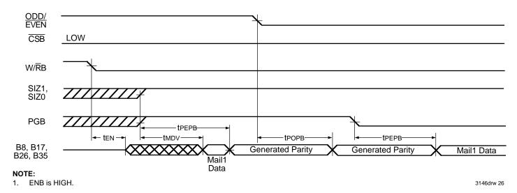
Figure 26. Parity Generation Timing when Reading from the Mail1 Register
