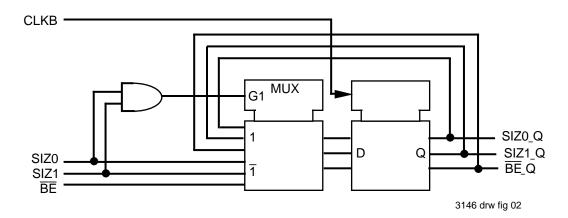
Figure 2. Logic Diagrams for SIZ0, SIZ1, and BE Register
