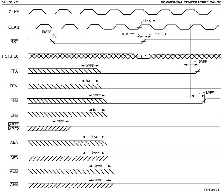
Figure 4. Device Reset Loading the X Register with the Value of Eight
