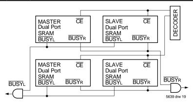
Figure 3. Busy and chip enable routing for both width and depth expansion with IDT70T35/34L (IDT70T25/24L) SRAMs.
