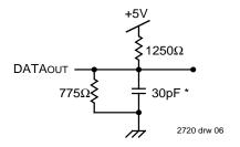
Figure 1. AC Output Test Load
