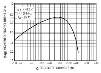
Figure 4. High Frequency Current Gain
