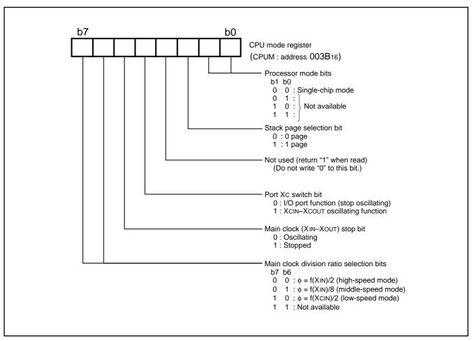
Fig. 5 Structure of CPU mode register
