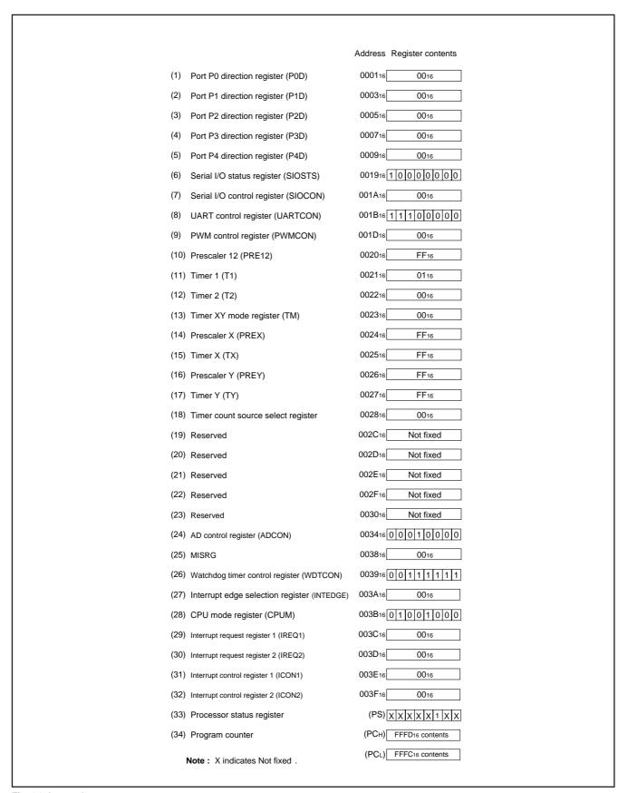
Fig. 31 Internal status at reset
