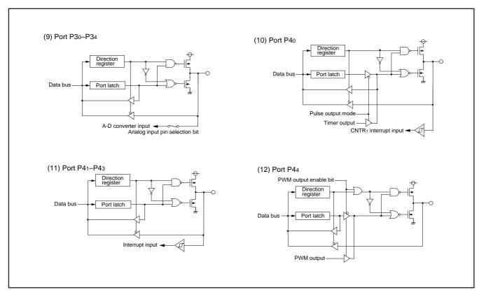
Fig. 9 Port block diagram (2)
