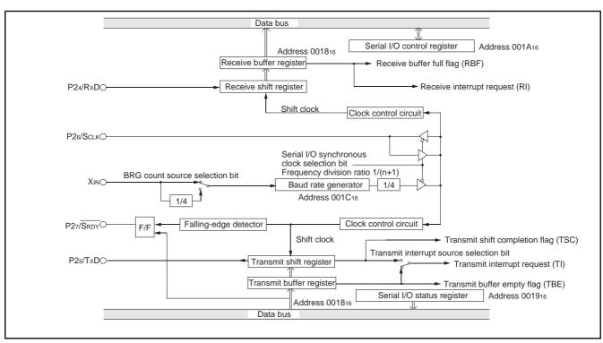
Fig. 15 Block diagram of clock synchronous serial I/O
