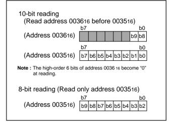
Fig. 25 Structure of A-D conversion registers
