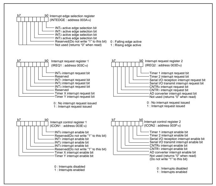
Fig. 11 Structure of interrupt-related registers (1)
