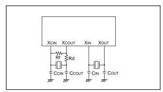
Fig. 32 Ceramic resonator circuit
