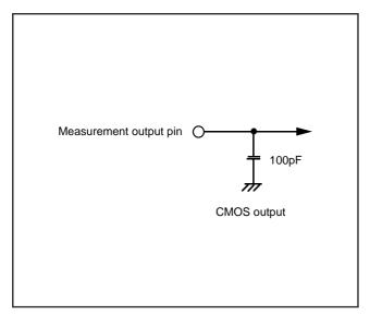
Fig. 38 Circuit for measuring output switching characteristics (1)
