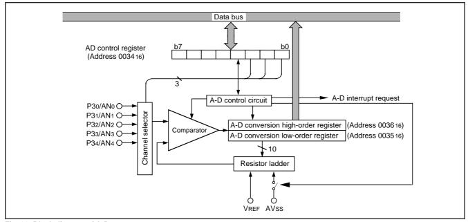
Fig. 26 Block diagram of A-D converter
