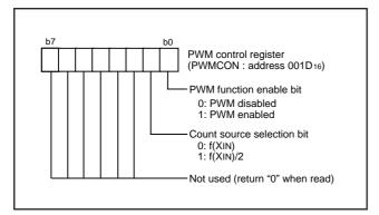
Fig. 22 Structure of PWM control register
