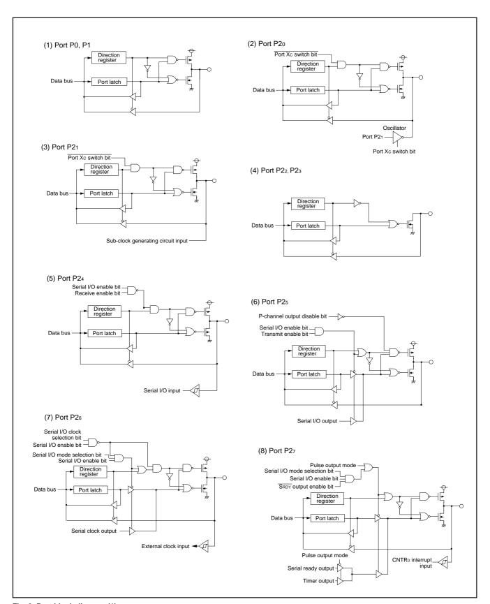
Fig. 8 Port block diagram (1)
