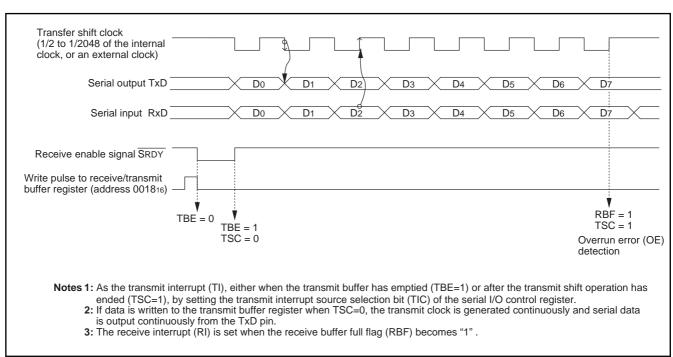
Fig. 16 Operation of clock synchronous serial I/O function
