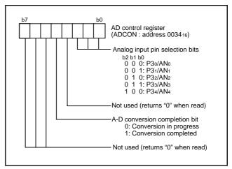
Fig. 24 Structure of AD control register
