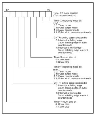
Fig. 12 Structure of timer XY mode register
