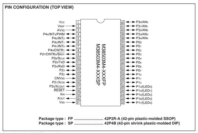
Fig. 1 M38503M4-XXXFP/SP pin configuration
