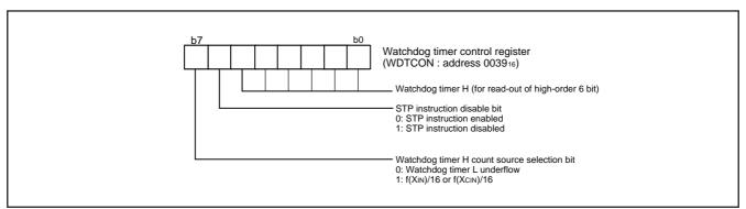
Fig. 28 Structure of Watchdog timer control register
