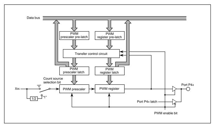
Fig. 21 Block diagram of PWM function
