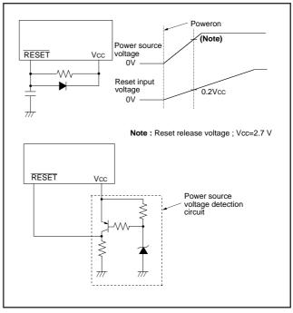
Fig. 29 Reset circuit example
