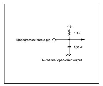
Fig. 39 Circuit for measuring output switching characteristics (2)
