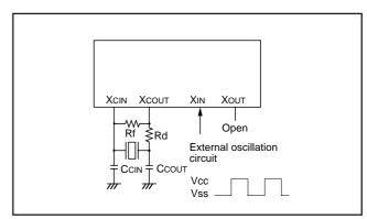
Fig. 33 External clock input circuit
