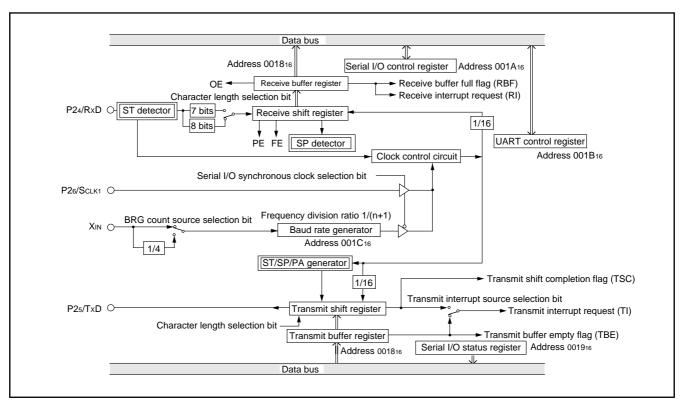
Fig.17 Block diagram of UART serial I/O
