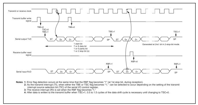
Fig. 18 Operation of UART serial I/O function
