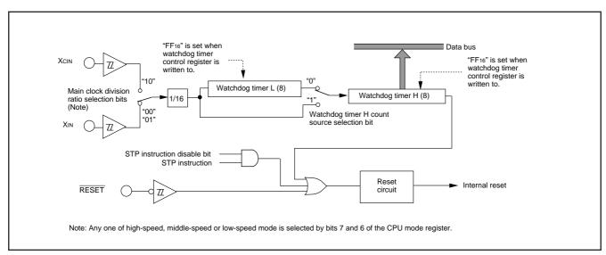
Fig. 27 Block diagram of Watchdog timer
