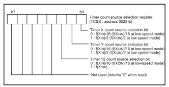
Fig. 13 Structure of timer count source selection register
