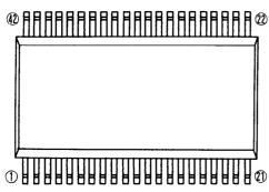
Note1: If the Special Mark is to be printed, indicate the desired layout of the mark in the left figure. The layout will be duplicated as close as possible. Mitsubishi lot number (6-digit or 7-digit) and Mask ROM number (3-digit) are always marked.
