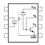
capability will enable the designer to interface any TTL family to CMOS. The availability of the base lead allows optimized gain/bandwidth adjustment in analog applications. The shallow depth of the IC photodiode provides better radiation immunity than conventional phototransistor couplers.
