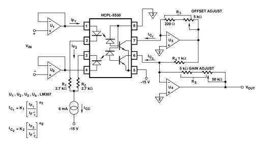
Figure 13. Isolation Amplifier Application Circuit.
