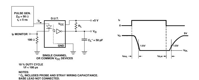
Figure 9. Switching Test Circuit.\*
