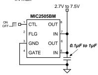
Figure 1. Supply Bypassing
