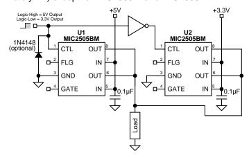
Figure 2. 5V/3.3V Switch Concept
