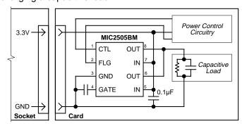
Figure 3. Hot Plug-In Concept
