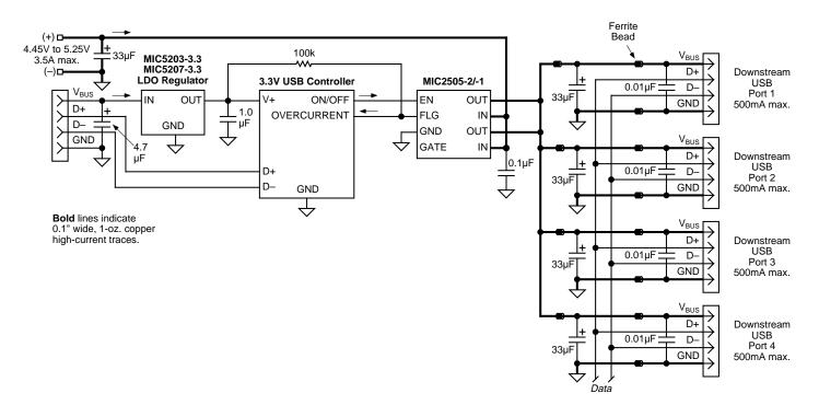
Figure 4. Ganged-Switch Self-Powered Hub
