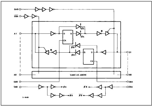
Note: In case of 74HCT652 output inverter marked \* at A bus and B bus are eliminated.
