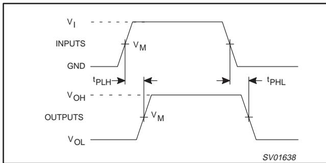
Figure 13. Input ( $V_{IS}$ ) to output ( $V_{Os}$ ) propagation delays.
