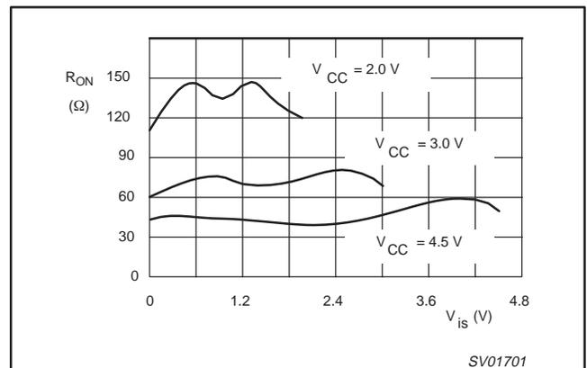
Figure 4. Typical ON-resistance (R<sub>ON</sub>) as a function of input voltage (V<sub>is</sub>) for V<sub>is</sub> = 0 to V<sub>CC</sub> - V<sub>EE</sub>.
