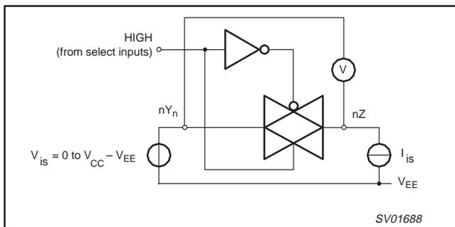
Figure 1. Test circuit for measuring ON-resistance (R<sub>ON</sub>).
