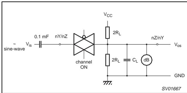
**Figure 10. Test circuit for measuring minimum frequency response.**
