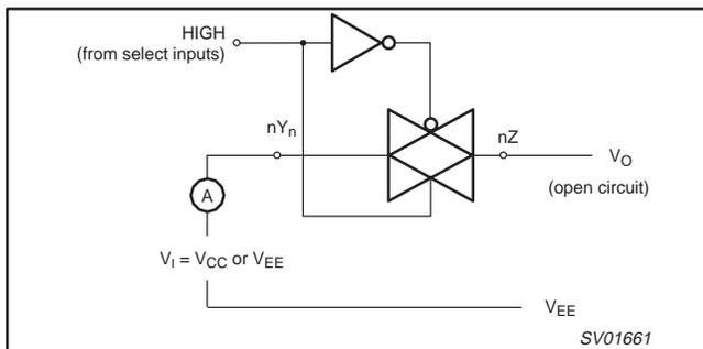
Figure 3. Test circuit for measuring ON-state current.
