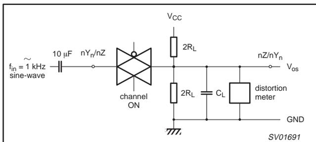
**Figure 11. Test circuit for measuring sine-wave distortion.**
