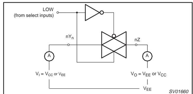
Figure 2. Test circuit for measuring OFF-state current.
