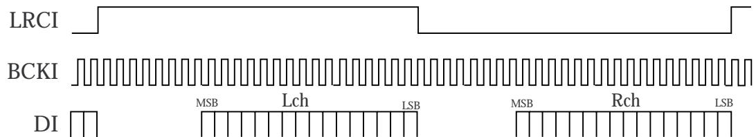
There must be a minimum of 16 BCKI clock cycles to read in a single word of data.
