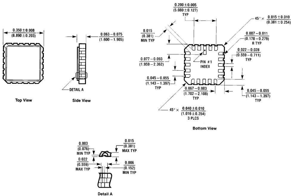
**20-Lead Ceramic Leadless Chip Carrier (L)
