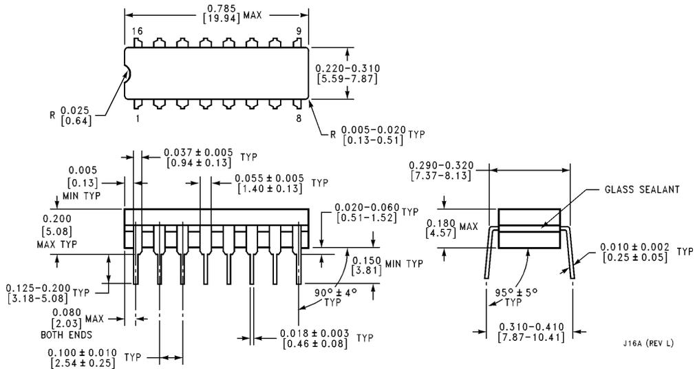
**16-Lead Ceramic Dual-In-Line Package (D)
