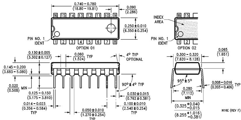
**16-Lead (0.300" Wide) Molded Dual-In-Line Package (P)
