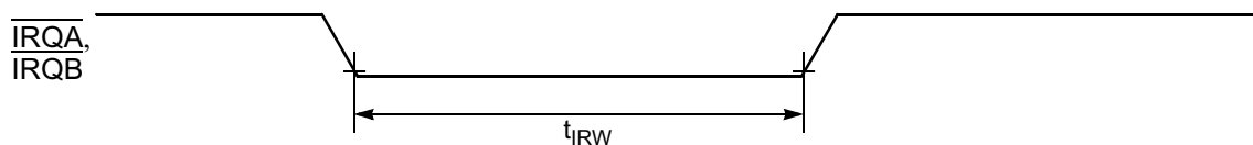
Figure 10-6 External Interrupt Timing (Negative Edge-Sensitive)
