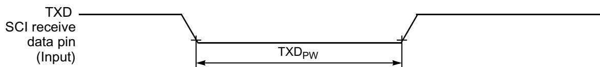
Figure 10-17 TXD Pulse Width
