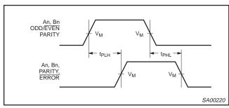
Waveform 2. Propagation Delay For Non-Inverting Output
