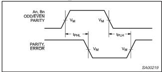
Waveform 1. Propagation Delay For Inverting Output
