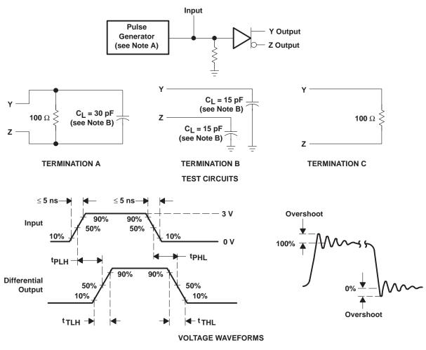
NOTES: A. The pulse generator has the following characteristics:  $Z_0 = 50 \ \Omega$ ,  $t_w = 25 \text{ ns}$ , PRR  $\leq 10 \text{ MHz}$ . B. CL includes probe and jig capacitance.
