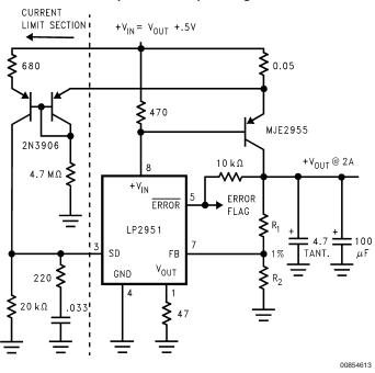
$V_{out} = 1.23V \left( 1 + \frac{R_1}{R_2} \right)$
