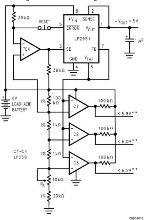
$^\star\textsc{Optional}$  Latch off when drop out occurs. Adjust R3 for C2 Switching when  $V_{in}$  is 6.0V.
