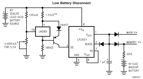
For values shown, Regulator shuts down when  $V_{in}$  < 5.5V and turns on again at 6.0V. Current drain in disconnected mode is  $\approx$  150 $\mu$ A. \*Sets disconnect Voltage
