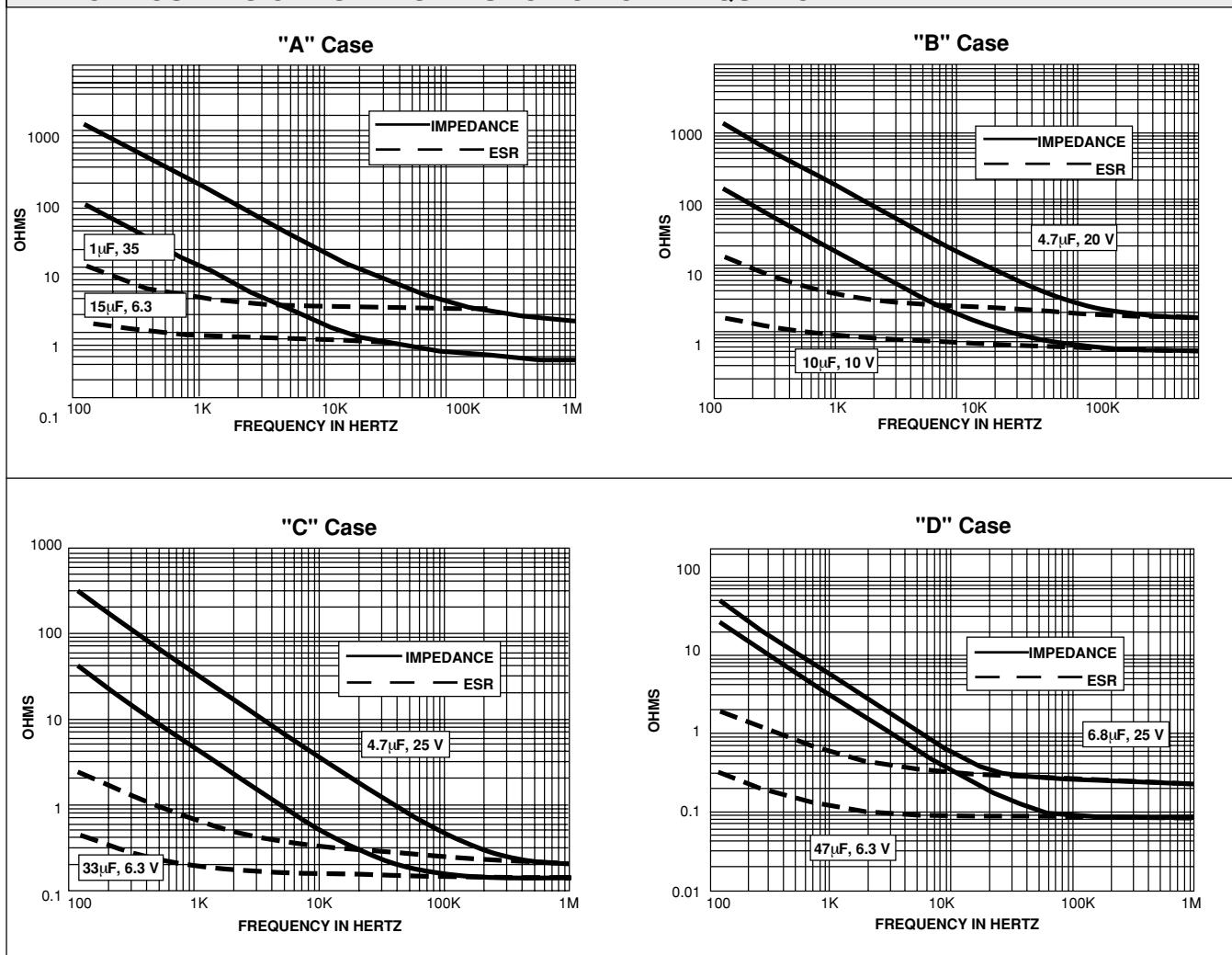
**TYPICAL CURVES @ + 25°C, IMPEDANCE AND ESR VS FREQUENCY**
