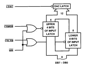
Figure 6. AD7248A Input Control Logic
