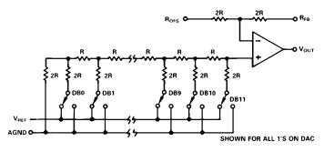
Figure 1. D/A Simplified Circuit Diagram
