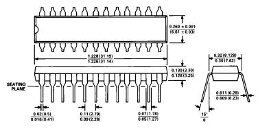
LEAD NO. 1 IDENTIFIED BY DOT OR NOTCH. PLASTIC LEADS WILL BE EITHER SOLDER DIPPED ON TIN LEAD PLATED IN ACCORDANCE WITH MIL-M-38510 REQUIREMENTS.
