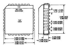
NOTES 'THIS DIMENSION CONTROLS THE OVERALL PACKAGE THICKNESS. 'APPLIES TO ALL FOUR SIDES. ALL TERMINALS ARE GOLD PLATED.
