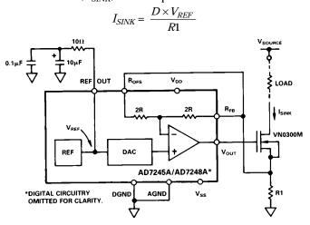
Figure 10. Programmable Current Sink
