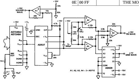
Figure 11. Programmable Function Generator
