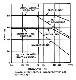
Power Supply Rejection Ration vs. Frequency
