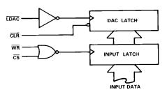
Figure 4. AD7245A Input Control Logic
