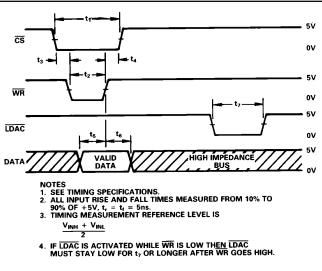
Figure 5. AD7245A Write Cycle Timing Diagram
