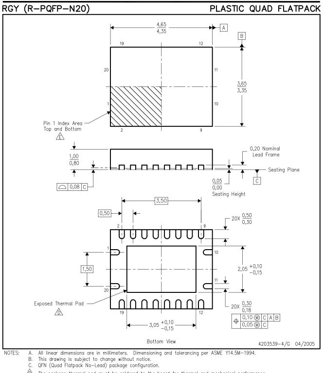
$\Delta$  The package thermal pad must be soldered to the board for thermal and mechanical performance.
