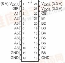
The SN74LVC4245A is designed for asynchronous communication between data buses. The device transmits data from the A bus to the B bus or from the B bus to the A bus, depending on the logic level at the direction-control (DIR) input. The output-enable ( $\overline{OE}$ ) input can be used to disable the device so the buses are effectively isolated.
