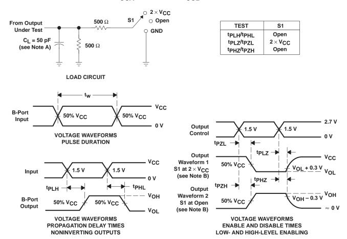
NOTES: A. C<sub>I</sub> includes probe and jig capacitance.
