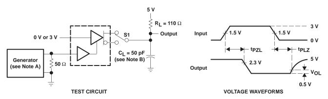
NOTES: A. The input pulse is supplied by a generator having the following characteristics: PRR = 1 MHz,  $Z_O = 50 \Omega$ , duty cycle = 50%,  $t_f \le 5$  ns.
