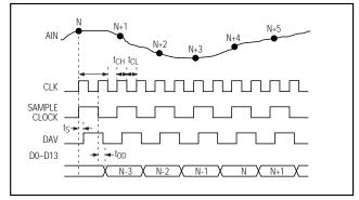
Figure 7. Main Timing Diagram
