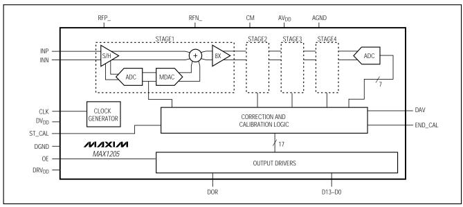
Figure 1. Internal Block Diagram
