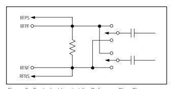
Figure 3. Equivalent Input at the Reference Pins. The sense pins should not draw any DC current.
