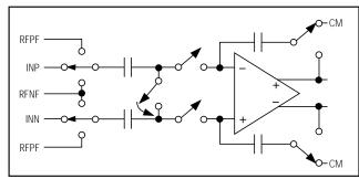
Figure 2. Simplified MDAC Architecture
