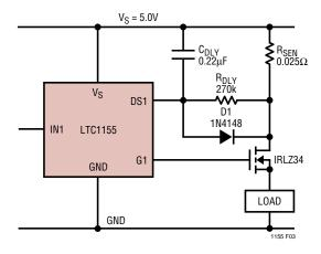
Figure 3. Using a Speed-Up Diode
