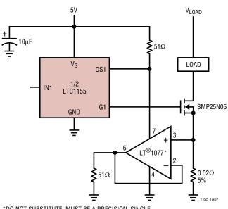
\*DO NOT SUBSTITUTE. MUST BE A PRECISION, SINGLE SUPPLY, MICROPOWER OP AMP (I  $_{\!Q} < 60 \mu A)$
