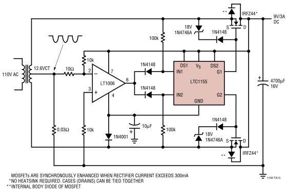
High Efficiency 60Hz Full-Wave Synchronous Rectifier
