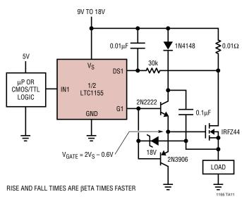
Logic Controlled Boost Mode Switching Regulator with Short-Circuit Protection and  $8\mu A$  Standby Current
