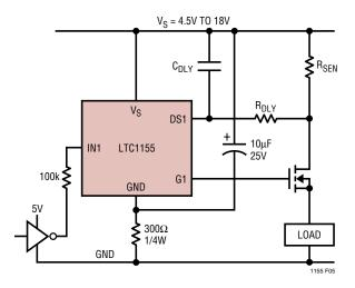
Figure 5. Reverse Battery Protection
