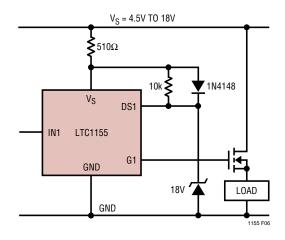
Figure 6. Overvoltage Shutdown and Protection
