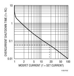
Figure 2. Shutdown Time vs MOSFET Current
