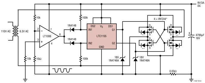
MOSFETS ARE SYNCHRONOUSLY ENHANCED WHEN RECTIFIER CURRENT EXCEEDS 300mA
