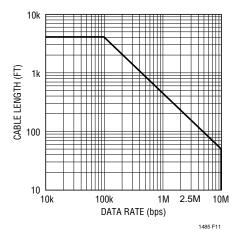
Figure 11. Cable Length vs Data Rate
