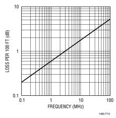
Figure 10. Attenuation vs Frequency for Belden 9481
