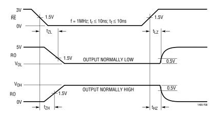
Figure 8. Receiver Enable and Disable Times
