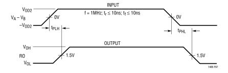
Figure 7. Receiver Propagation Delays
