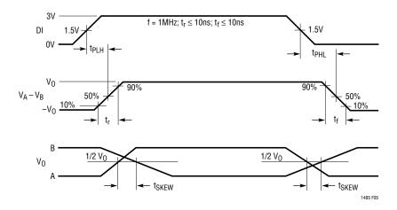
Figure 5. Driver Propagation Delays
