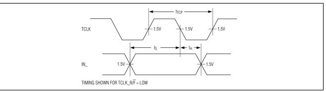
Figure 5. Data Input Setup and Hold Times
