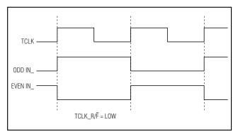
Figure 2. Worst-Case ICC Test Pattern
