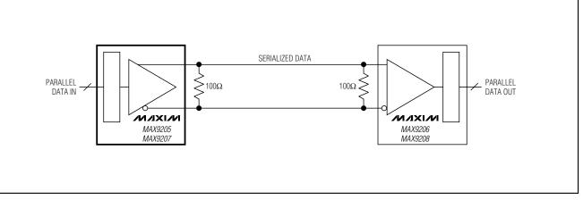
Figure 11. Double-Terminated Point-to-Point
