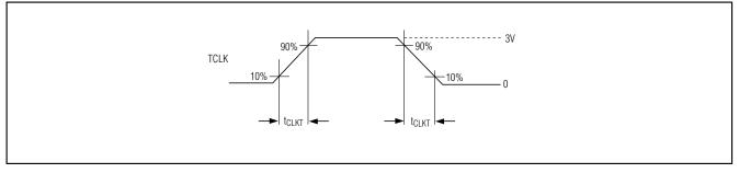
Figure 3. Input Clock Transition Time Requirement
