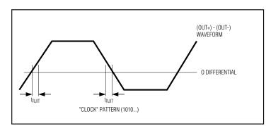
Figure 10. Definition of Random Jitter (t<sub>RJIT</sub>)
