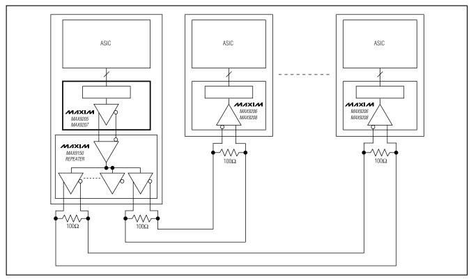
Figure 13. Point-to-Point Broadcast Using MAX9150 Repeater
