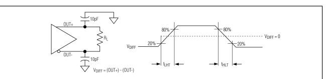
Figure 4. Output Load and Transition Times
