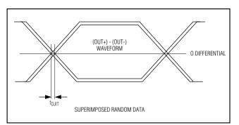
Figure 9. Definition of Deterministic Jitter (t<sub>DJIT</sub>)
