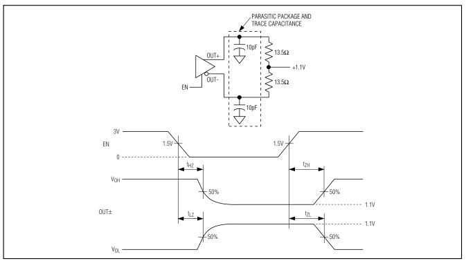
Figure 6. High-Impedance Test Circuit and Timing
