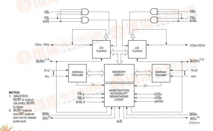
RAM for 16-bit-or-more word systems. Using the IDT MAS-TER/SLAVE Dual-Port RAM approach in 16-bit or wider memory system applications results in full-speed, error-free operation without the need for additional discrete logic.
