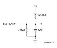
Figure 1. AC Output Test Load
