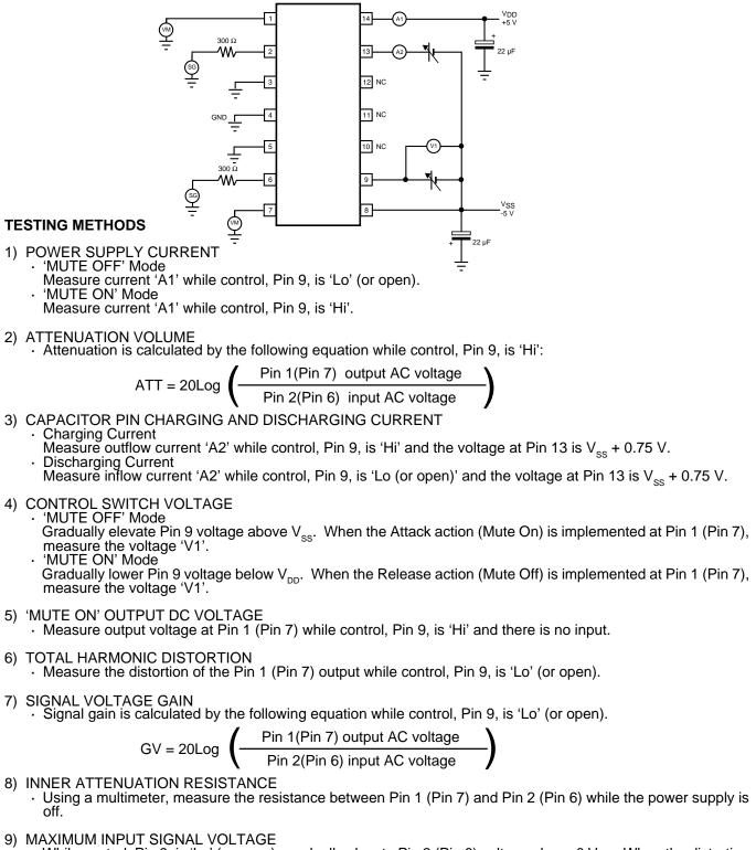
While control, Pin 9, is 'Lo' (or open), gradually elevate Pin 2 (Pin 6) voltage above 0 V<sub>P.P</sub>. When the distortion becomes 0.01% at the output of Pin 1 (Pin 7), measure the AC voltage.
