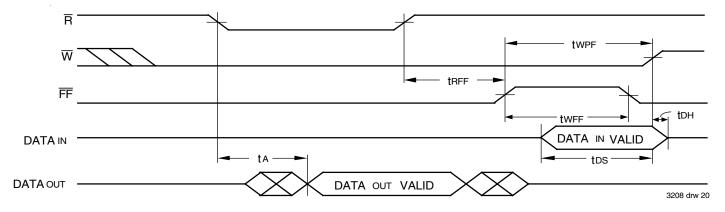
Figure 18. Write Data Flow-Through Mode
