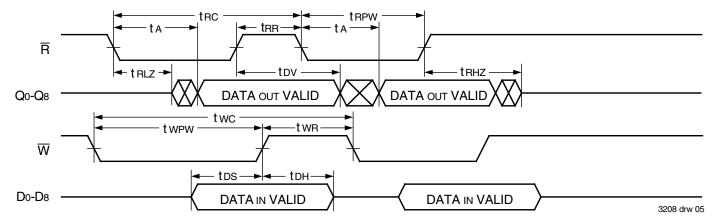
Figure 3. Asynchronous Write and Read Operation
