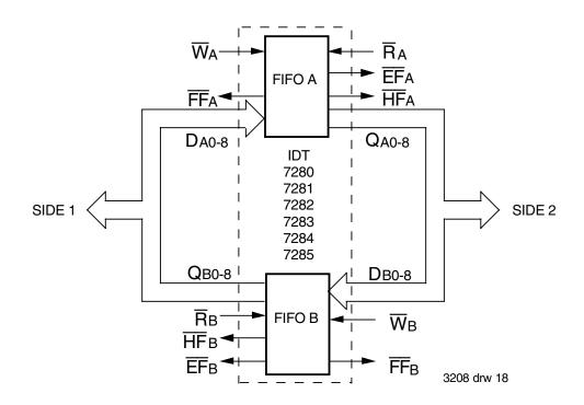
Figure 16. Bidirectional FIFO Mode
