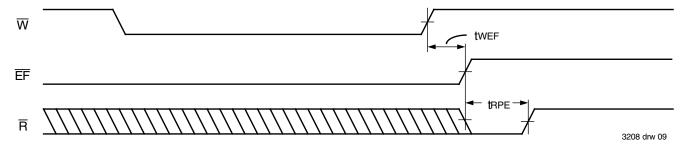
Figure 7. Minimum Timing for an Empty Flag Coincident Read Pulse
