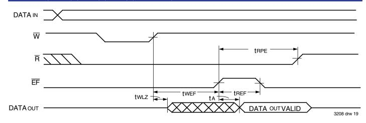
Figure 17. Read Data Flow-Through Mode
