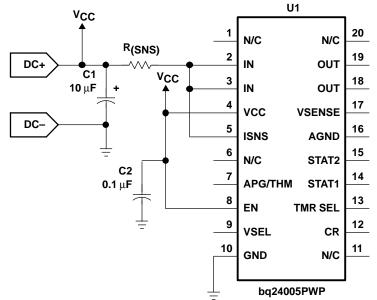
Figure 19. Current Sensing Circuit
