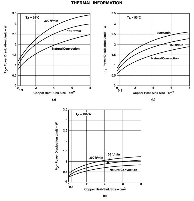
Figure 22. Power Ratings of the PWP Package at Ambient Temperatures of 25°C, 55°C, and 105°C
