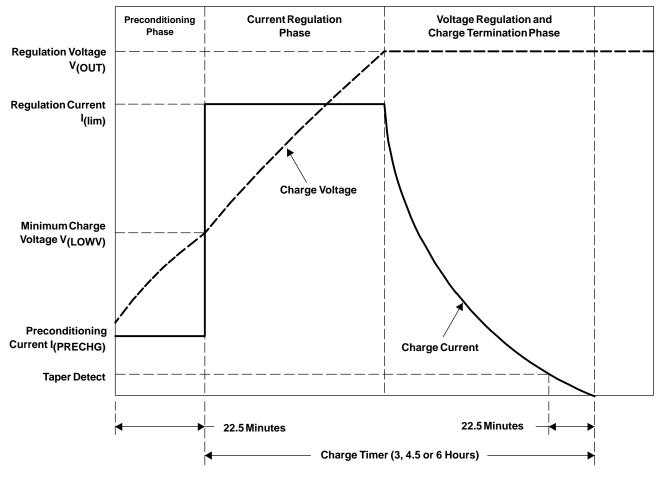
Figure 14. Typical Charge Profile
