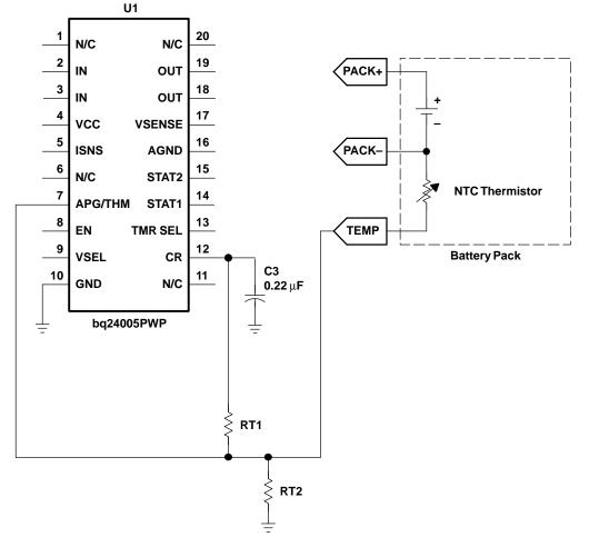
Figure 16. Temperature Sensing Circuit
