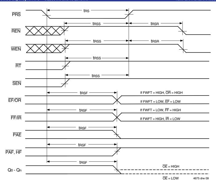
Figure 6. Partial Reset Timing
