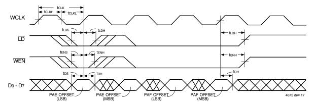
Figure 14. Parallel Loading of Programmable Flag Registers (IDT Standard and FWFT Modes) for the IDT72281
