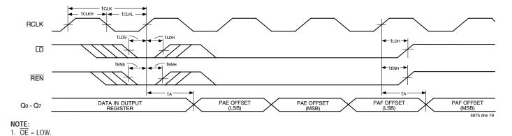
Figure 16. Parallel Read of Programmable Flag Registers (IDT Standard and FWFT Modes) for the IDT72281
