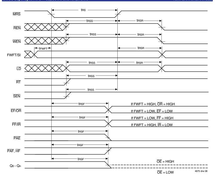
Figure 5. Master Reset Timing
