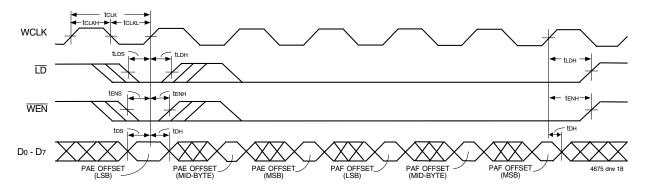
Figure 15. Parallel Loading of Programmable Flag Registers (IDT Standard and FWFT Modes) for the IDT72291
