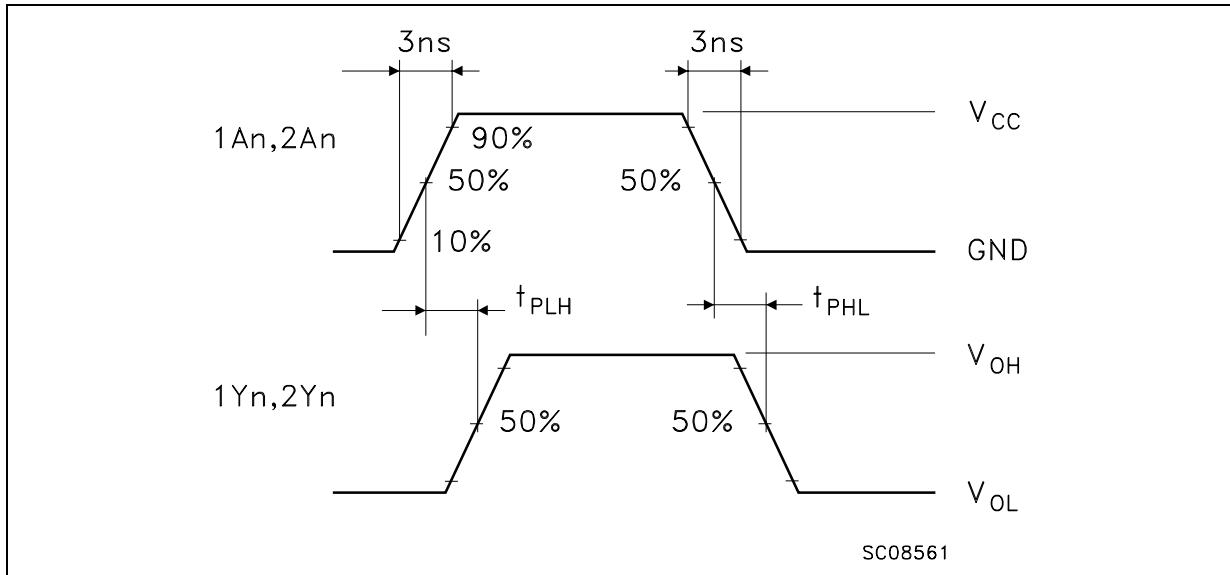
**WAVEFORM 2: OUTPUT ENABLE AND DISABLE TIME (f=1MHz; 50% duty cycle)**
