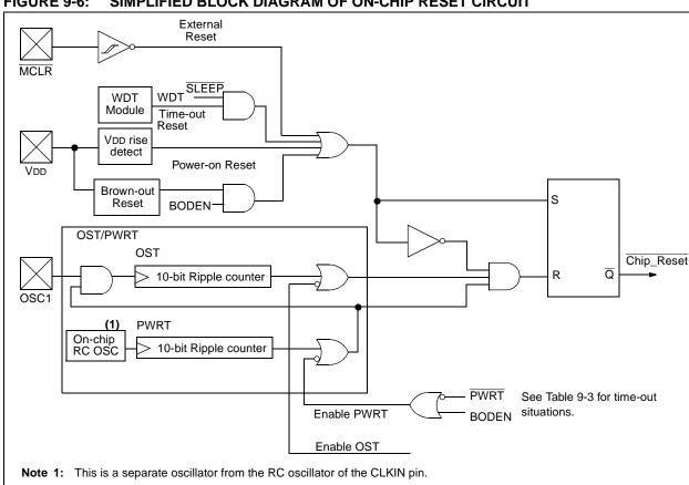
FIGURE 9-6: SIMPLIFIED BLOCK DIAGRAM OF ON-CHIP RESET CIRCUIT
