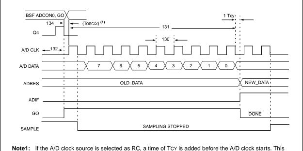
Note1: If the A/D clock source is selected as RC, a time of Tcy is added before the A/D clock starts. This allows the SLEEP instruction to be executed.
