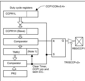
Note 1: 8-bit timer is concatenated with 2-bit internal Q clock or 2 bits of the prescaler to create 10-bit time-base.
