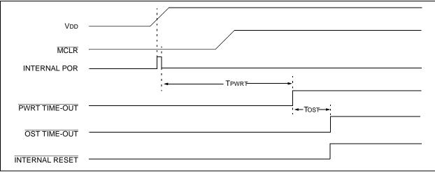
FIGURE 9-13: TIME-OUT SEQUENCE ON POWER-UP (MCLR NOT TIED TO VDD): CASE 2
