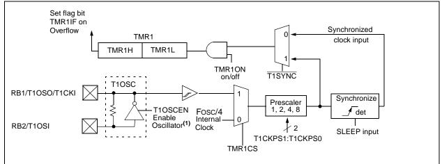
Note 1: When the T1OSCEN bit is cleared, the inverter and feedback resistor are turned off. This eliminates power drain.
