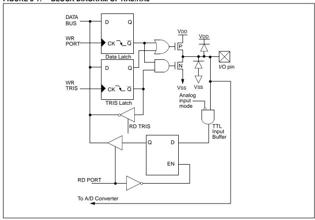
FIGURE 3-2: BLOCK DIAGRAM OF RA4/T0CKI PIN
