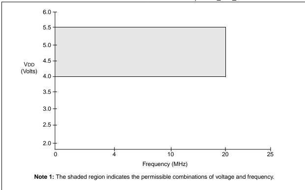
FIGURE 12-2: PIC16LC712/716 VOLTAGE-FREQUENCY GRAPH, 0°C ≤ TA ≤ +70°C
