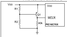
Note 1: This brown-out circuit is less expensive, albeit less accurate. Transistor Q1 turns off when VDD is below a certain level such that:
