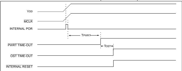
FIGURE 9-12: TIME-OUT SEQUENCE ON POWER-UP (MCLR NOT TIED TO VDD): CASE 1
