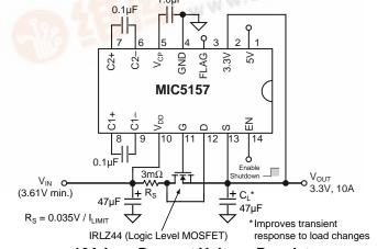
10A Low-Dropout Voltage Regulator
