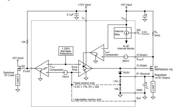
Block Diagram with External Components Fixed 3.3V Power Supply with 5.0V Load Switch
