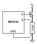
Figure 1a. Connections for Fixed Output
