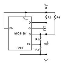
Figure 5. Battery Charger Concept
