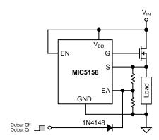
Figure 4b. Fast High-Side Switch
