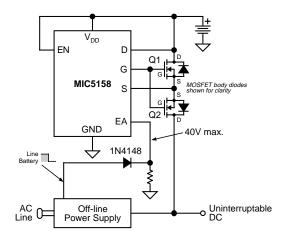
Figure 6. UPS Power Supply Concept
