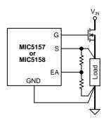
Figure 1b. Connections for Adjustable Output
