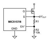
Figure 2. Typical Resistive Divider
