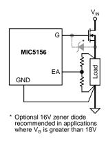
Figure 1c. MIC5156 Connections for Adjustable Output
